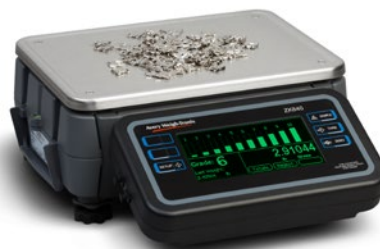
70 lb (35 kg) model 9 in x 12 in (230 mm x 305 mm) platter
